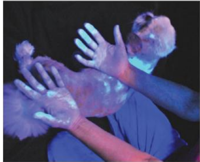
Fig. 3. Handling of a dog treated with Frontline ® containing 1% Tinopal ® CBS-X fluorescent tracer revealed contamination of hands during routine application and handling of a treated dog (color figure available online).
